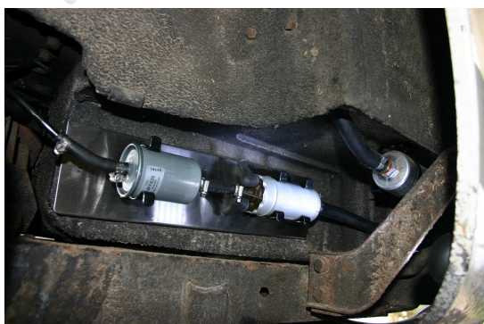
Fuel pump and filters
